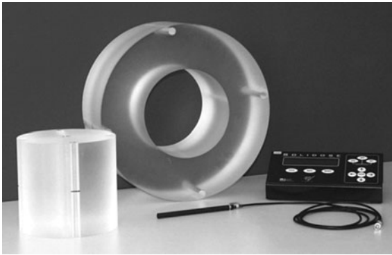
Fig. 2 Cylindrical standard CT dosimetry phantoms made from Perspex. The phantoms with a diameter of 16 cm and 32 cm are used for representative CTDI measurements of the head and trunk, respectively. For dose measurement the pencil ionization chamber with an active length of 100 mm is inserted into the holes
